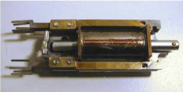
Fig. Electromechanical relays, similar to the 1950's phone relay shown here, were used in some early computing devices before vacuum tubes became more popular. (da http://www.computermuseum.li/Testpage/Relay1950.htm )
